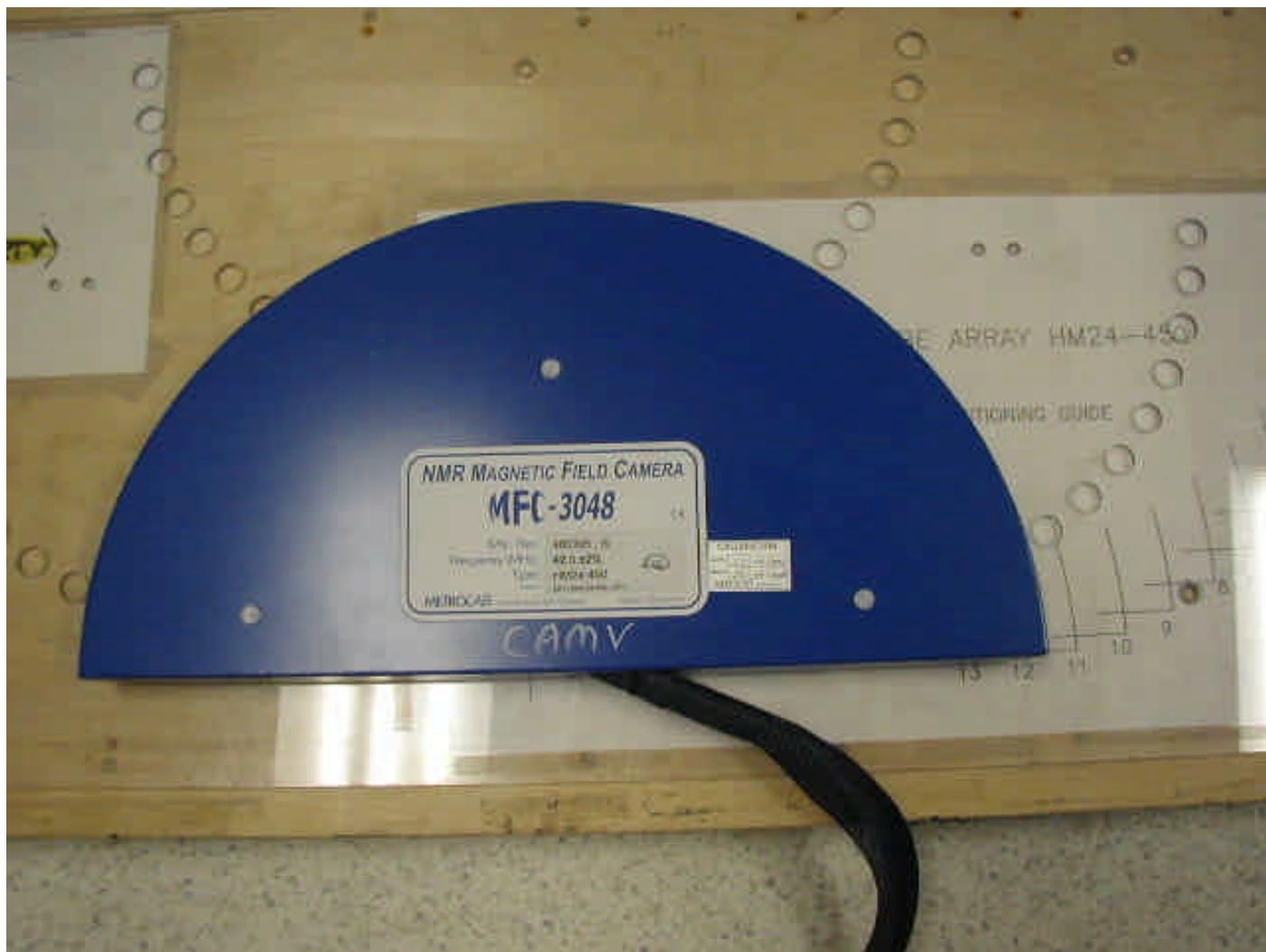
Figure 1: Probe Array resting in the middle position on the normalization jig.
