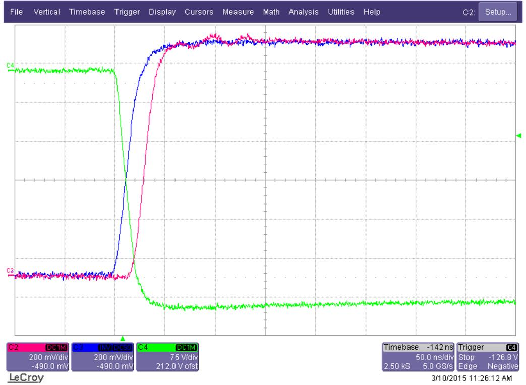
Ch 1: Co-ax shunt, DC-800MHz – 200mV/div (2A/div)
