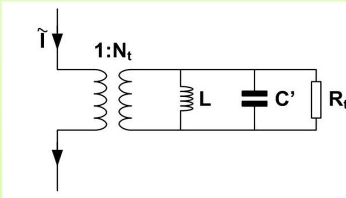
The insertion impedance is a parallel combination of  $L_1$ ,  $C_1$ ,  $R_1$ , where
