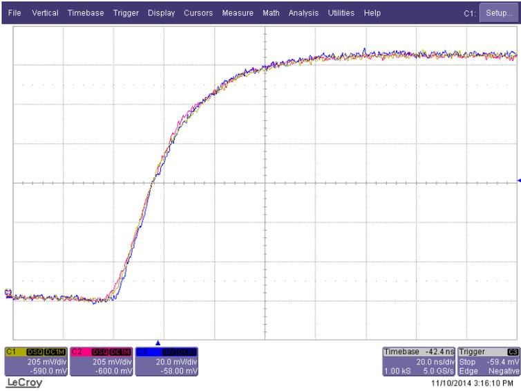
**Ch 1: Co-ax shunt, DC-800MHz – 20mV/div**
