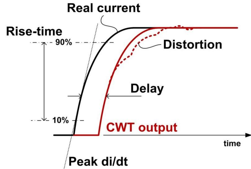
The CWT has an inherent measurement **delay**. Provided the rise-time of the current is within the limits of the high frequency bandwidth (termed **Max. rise-time**) of the CWT the delay is predictable.
