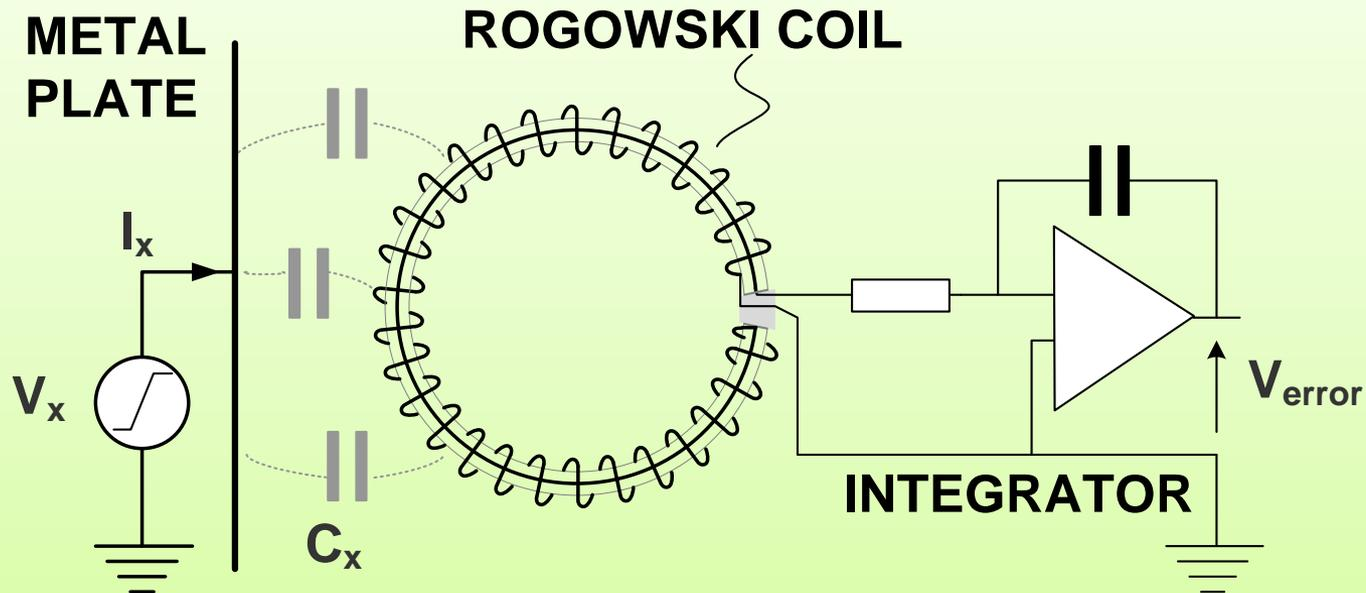
A disturbance  $dV_x/dt$  causes an unwanted displacement current to flow onto the coil winding ultimately giving rise to interference  $V_{error}$
