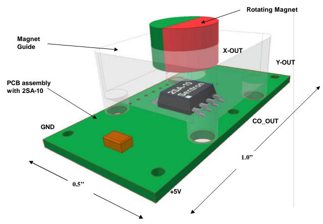
Outputs can be measured between Y-OUT,  $X_OUT$  and CO-OUT for a differential output or between Y-OUT,  $X_OUT$  and GND for single ended output. Apply regulated +5 volts between the +5V and GND terminals. Magnet and Guide are optimized to provide a 2.5 +/- 0.2 volt at the X-OUT and Y-OUT outputs. As the magnet is rotated 360 degrees, the X and Y outputs will generate a SIN and COSINE voltage at the X and Y outputs respectively
