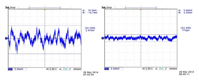
The majority of the noise is very low frequency and is centred on the low frequency bandwidth, which is 0.45Hz for the LFR03/3.
