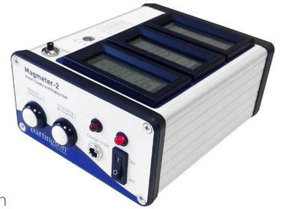
Low-pass filtering (9.5kHz) is applied to all inputs in order to prevent the excitation signal of the fluxgate sensor from affecting the measurement, while a high-pass filter (0.1Hz) is selectable via a front panel switch when AC measurements are preferred. The unit is compatible with most differential or single-ended sensors from Bartington Instruments. The internal batteries are recharged when the unit is connected to mains power using the adaptor provided.
