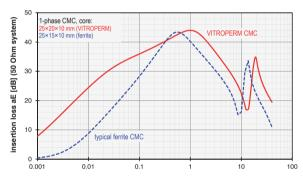
Fig. 5: Comparison of insertion loss of VITROPERM and ferrite
