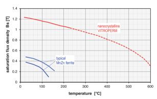
Fig. 9: Temperature dependence of saturation flux density B<sub>s</sub>(T)
