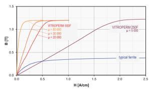
Fig. 8b: Magnetization curve of VITROPERM 500 F and VITROPERM 250 F in comparison to typical MnZn ferrite, showing noticeable differences in permeability (slope of the curve) and saturation flux density (B<sub>c</sub>)
