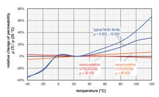
Fig. 10: Relative change of  $\mu(T)$  at f=100 kHz, normalized for room
