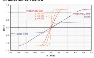
Fig. 8a: Hysteresis loops for various types of VITROPERM and typical MnZn ferrite
