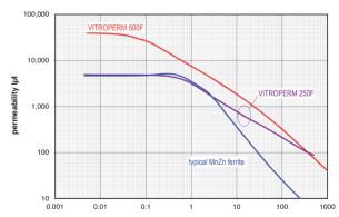
Fig. 6: Frequency response of the permeability of VITROPERM 500 F  $(\mu = 40,000)$  and VITROPERM 250 F  $(\mu = 5,000)$  in comparison to a typical MnZn ferrite ( $\mu = 5,000$ )
