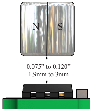
Air Gap Operating Range for the 55B0081 Cylindrical Magnet
