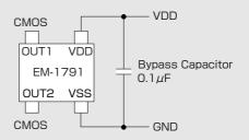
The characteristics with  $\lceil * \rfloor$  marks are design targets. OUT1 responds to the positive flux from the south pole(Bop1,Brp1),OUT2 to the
