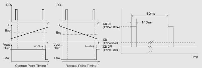
This Hall IC's output is held as internal data just before the internal circuit turns OFF (IDD OFF). And after 48.8  $\mu$ s, the output changes. Note) 48.8  $\mu$ s in figures is typical value
