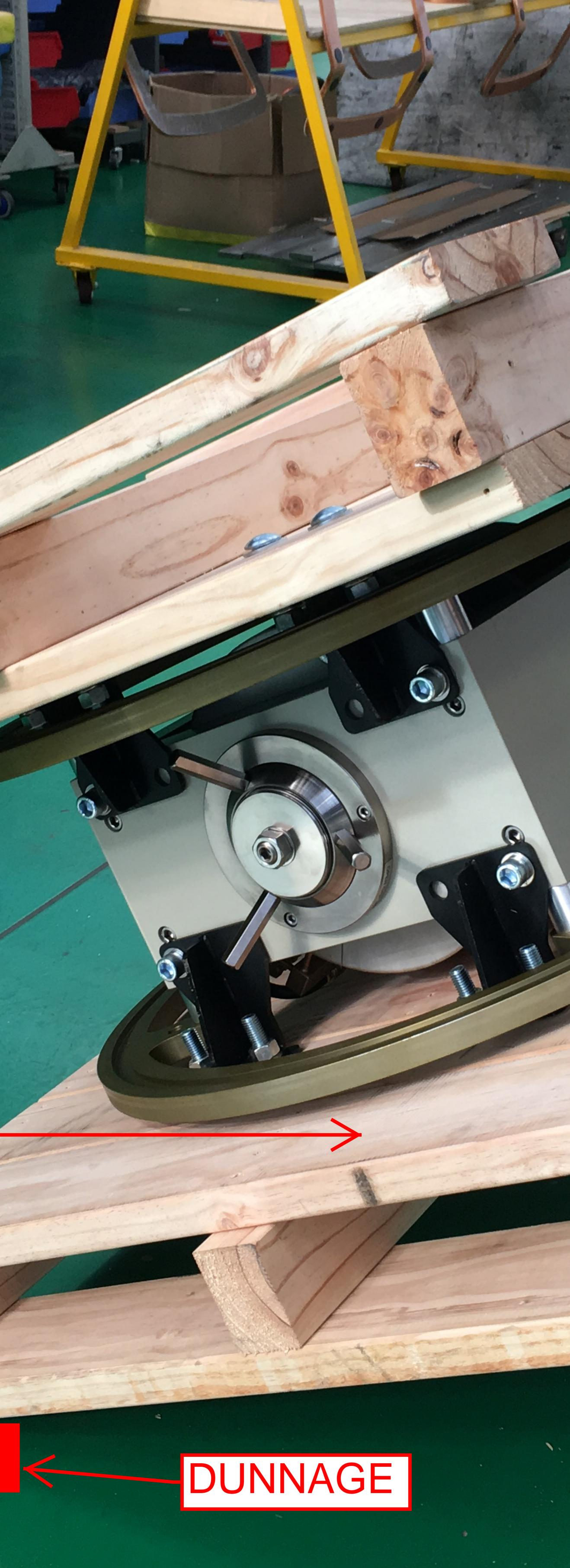
6. Slowly raise the crate to rotate the magnet through 90°. NOTE: TAKE CAUTION OF THE CRATE SWINGING WHEN THE CENTRE OF GRAVITY PASSES THE PIVOT EDGE. Swing can be mitigated using dunnage on the right hand side of the pivot edge. 7. Lower the crate so that the pallets rest on the ground.
