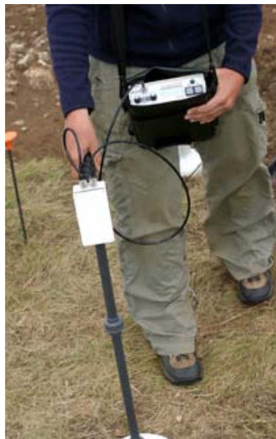
Fig.3. The MS2D field sensor in use
