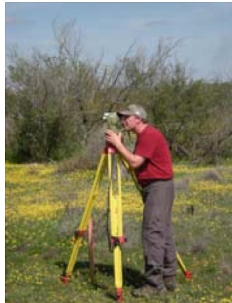
The time of each measurement is recorded. The four angular measurements are used to find the horizontal field position H. Using the known reference previously measured, the declination angle D can be calculated.
