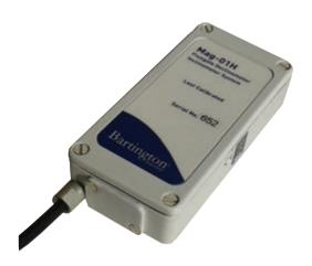
The Mag A probe contains a fluxgate element selected for high rejection of orthogonal fields. The element is extremely high quality, very stable and well aligned with little offset. The probe alignment will normally be stable to 1 minute of arc over the suggested two-year calibration period. Re-adjustment is seldom required.
