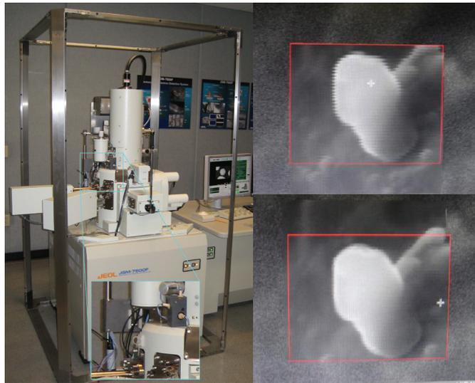
**Figure 1.** The left hand image shows a typical Mag-NetX installation with Mag-03IE70v1 sensor. In the top right image the B field is not suppressed. In the bottom right it is suppressed with the Mag-NetX system. Scanning Electron Microscope, Magnification 70k.
