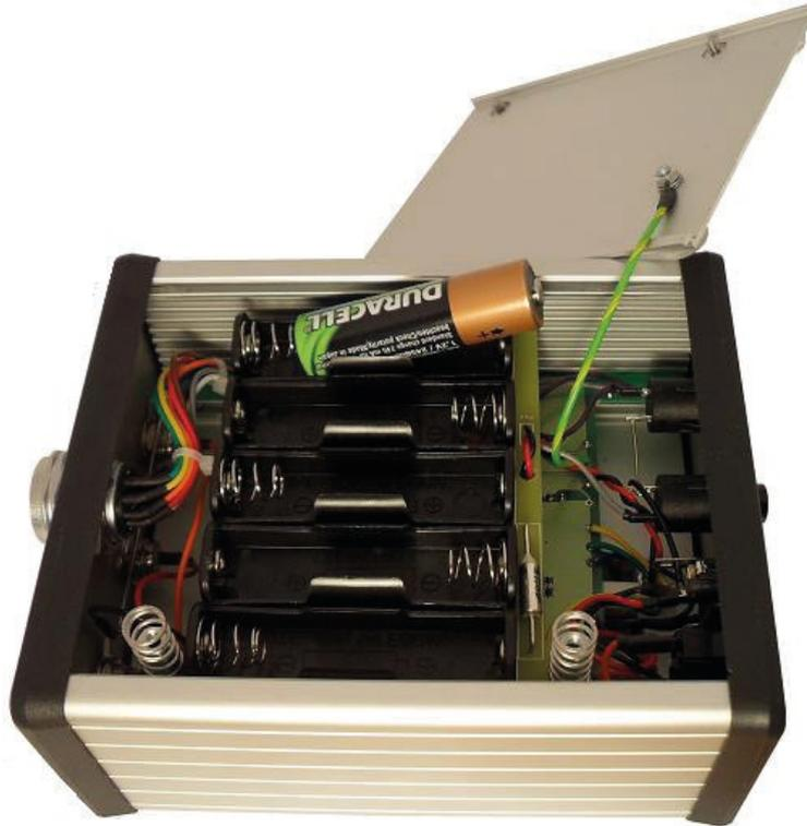
Insert each cell into the compartment in turn.
