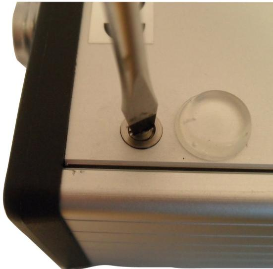
Fully loosen screw B and the lid of the enclosure will lift due to the internal springs.
