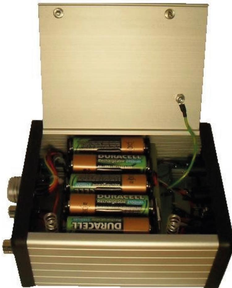
When all 5 cells are in place, locate the back edge of the lid in the enclosure.
