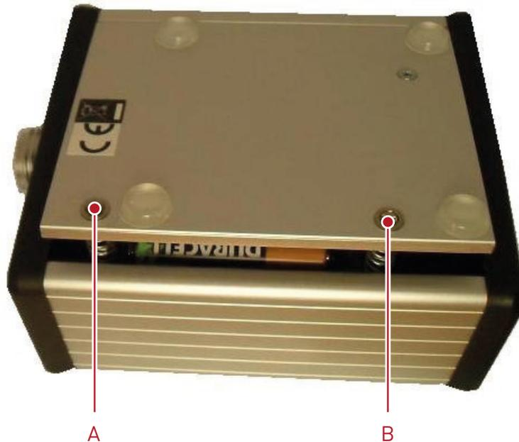
Tighten screws A and B in any order.
