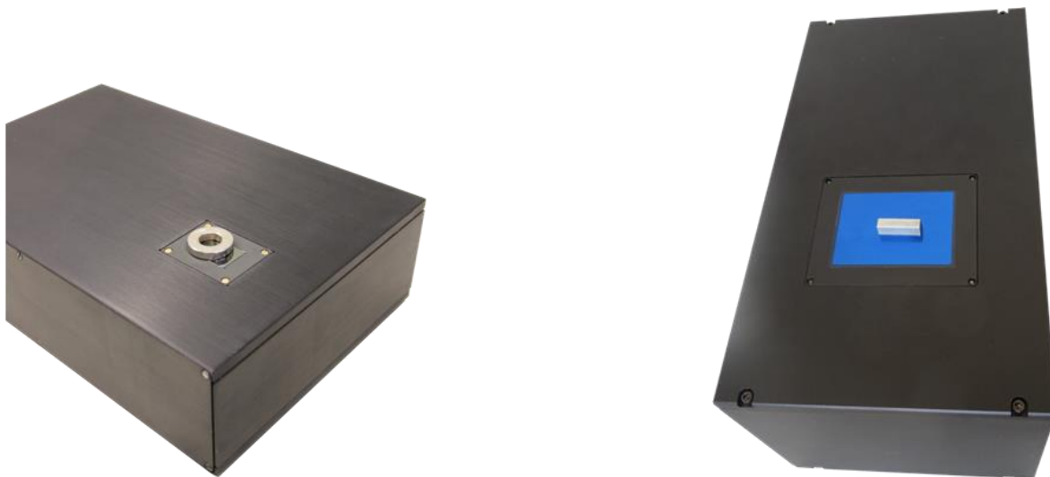
Figure 2: 1" and 3" CMOS-Magview, top view, each with specimen mounted on sensor.
