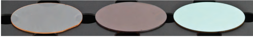
Fig. 2 — Magneto-optical (MO) sensors in various manufacturing stages: (from left to right) initial substrate, coated with MO layer, coated with reflective layer.
