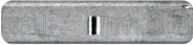
Fig. 8 — Magnetooptical recording of a mono audio tape showing a clearly visible “erasing” imprint by the writing-head and deleted sector; track height = 3 mm.
