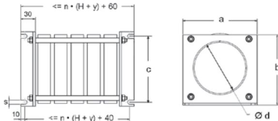
Dimensions of the core stack assemblies
