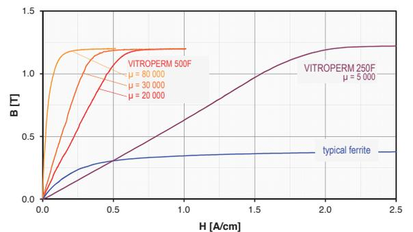
Fig. 8b: Magnetization curve of VITROPERM 500 F and VITROPERM 250 F in comparison to typical MnZn ferrite, showing noticeable differences in permeability (slope of the curve) and saturation flux density ( $B_s$ )
