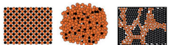
Fig 2: Crystalline structure, amorphous structure, nanocrystalline micro-structure
