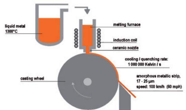
Fig. 1: Rapid solidification technology is used to produce thin metal tapes with an amorphous structure (metallic glass).
