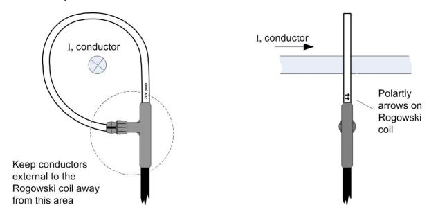
The sensitivity of the RCT1A to currents that do not pass through the coil is very small, provided that such currents are no greater than the RCT1A rating or such currents are relatively distant from the coil. In the vicinity of a multi-turn inductor the 'H' field is far stronger than from a single conductor carrying the same current, and such positions should be avoided.
