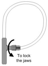
The locking mechanism must not be actuated at temperatures below 0°C
