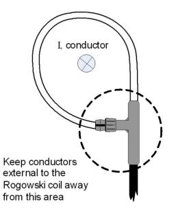
The sensitivity of the RCTrms to currents that do not pass through the coil is very small, provided that such currents are no greater than the RCTrms rating or such currents are relatively distant from the coil. In the vicinity of a multi-turn inductor the 'H' field is far stronger than from a single conductor carrying the same current, and such positions should be avoided.
