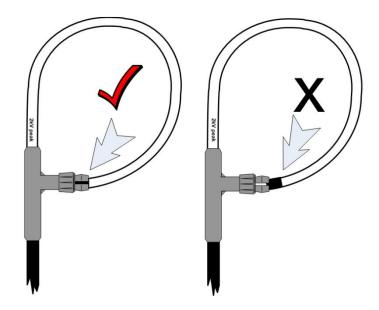
If the coil is to be left in-situ for any period of time or is used in an environment where the coil is subject to vibration the locking nut should be engaged as shown in the diagram below.
