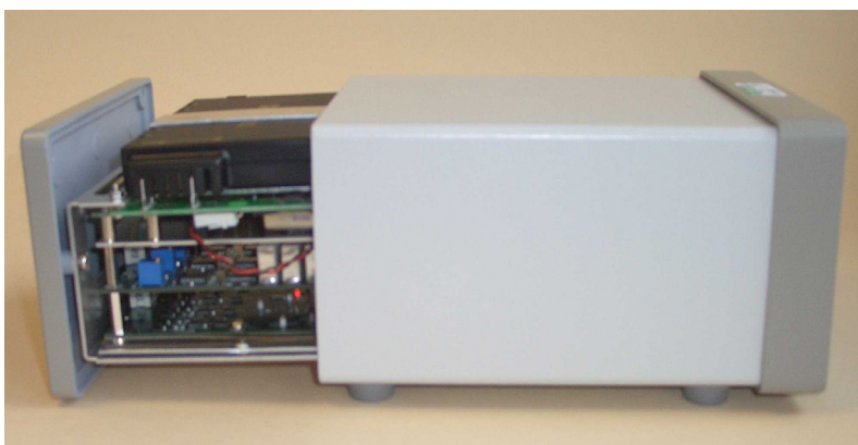
Figure 24a: Internal battery location.
