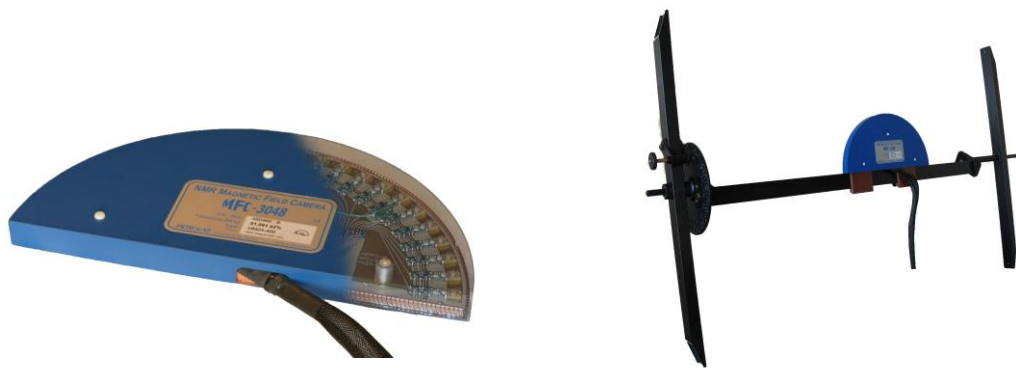
Figure 4. The Magnetic Field Camera probe array: (a) cut-away showing the probe positions; (b) as installed in a horizontal MRI magnet.
