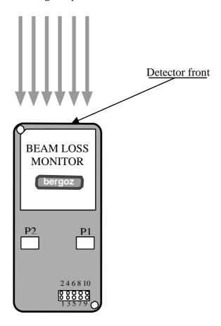
Mathematical simulation would indicate where beam loss is most likely to occur (See Annex I for FODO structure beam loss). BLMs will generally be placed with the front applied against the magnets.
