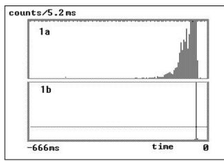
Figure 1: The last 666 ms before beam abort versus loss rate (arb. units) of a BLM in HERAp. One line represents the count rate integrated over 5.2 ms. The threshold is represented by a horizontal line. 1a: normal increase of the loss rate due to RF drop. 1b: very fast beam loss. The time of the beam dump is indicated by the fast decrease of the rate near t=0.
