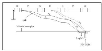
Figure 3: Path of electrons with by L defined energy losses after Bremsstrahlung at different locations (not in scale).  $e_{1,3}$  and  $e_{2,4}$  represents  $e_{min}$  and  $e_{max}$ .
