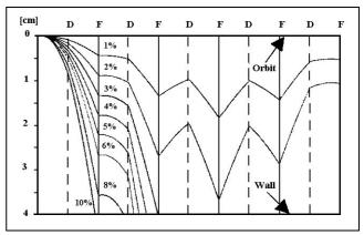
Figure 2: Path of electrons after energy losses. The deviation from the nominal energy is given in %. The vacuum wall starts at 4 cm in HERAe.
