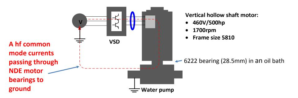
The Rogowski coil is positioned around all three phase terminal leads. In this position the Rogowski coil will measure the high frequency currents which were not returning to the inverter through the terminal leads (common mode currents).
