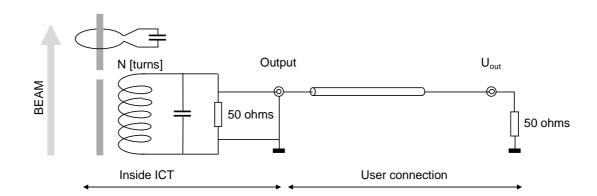
The ICT is a capacitively shorted transformer coupled to a fast readout transformer in a common magnetic circuit<sup>2</sup>.
