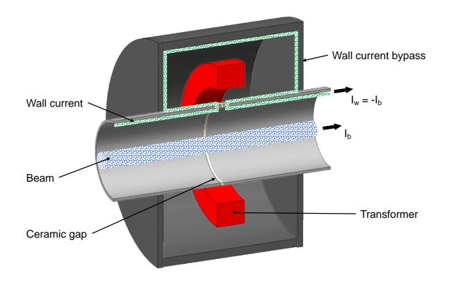
The transformer "sees" the wall current I<sub>w</sub>. The higher frequencies of the wall current frequency spectrum will pass thru the capacitance of the ceramic gap, while the lower frequencies will enter the cavity and induce a flux in the transformer core.
