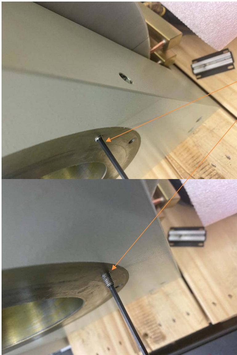
The side retaining ring must be removed prior to removing the set screw shown. Use an M3 allen wrench to remove the set screw.
