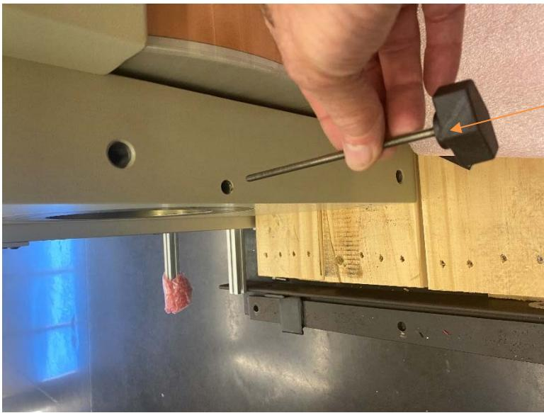
Once the set screw is removed use the tool provided with the new poles to pull the hard stop pin.
