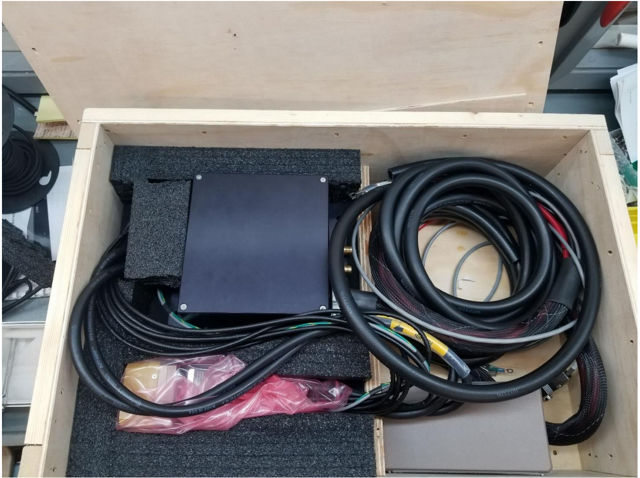
Figure 1: Shown here is packing configuration for the magnet head, the junction box and the electrical cable. These are all connected and ready to install. Also included is 5m of water hose, not connected, and four hose clamps.
