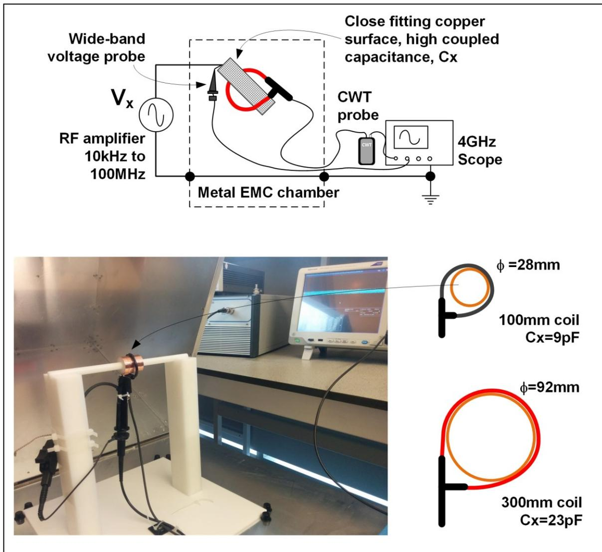
Figure 2. Test set-up for determining voltage immunity
