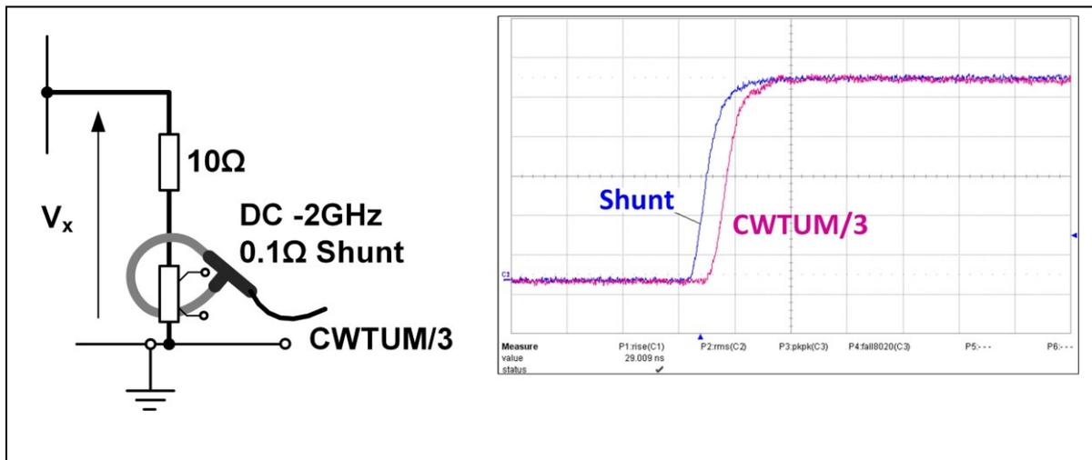
**Figure 6. Measurement of 30ns rise-time 50A at the 'quiet' earthed end of the circuit
