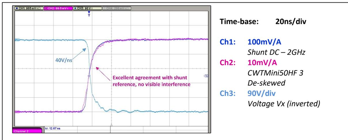
Figure 5. Measurement of 12ns / 50A current transient with local  $dV/dt$  40V/ns
