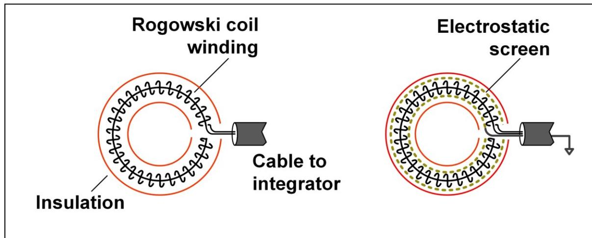
Figure 1. Screened and Unscreened coils
