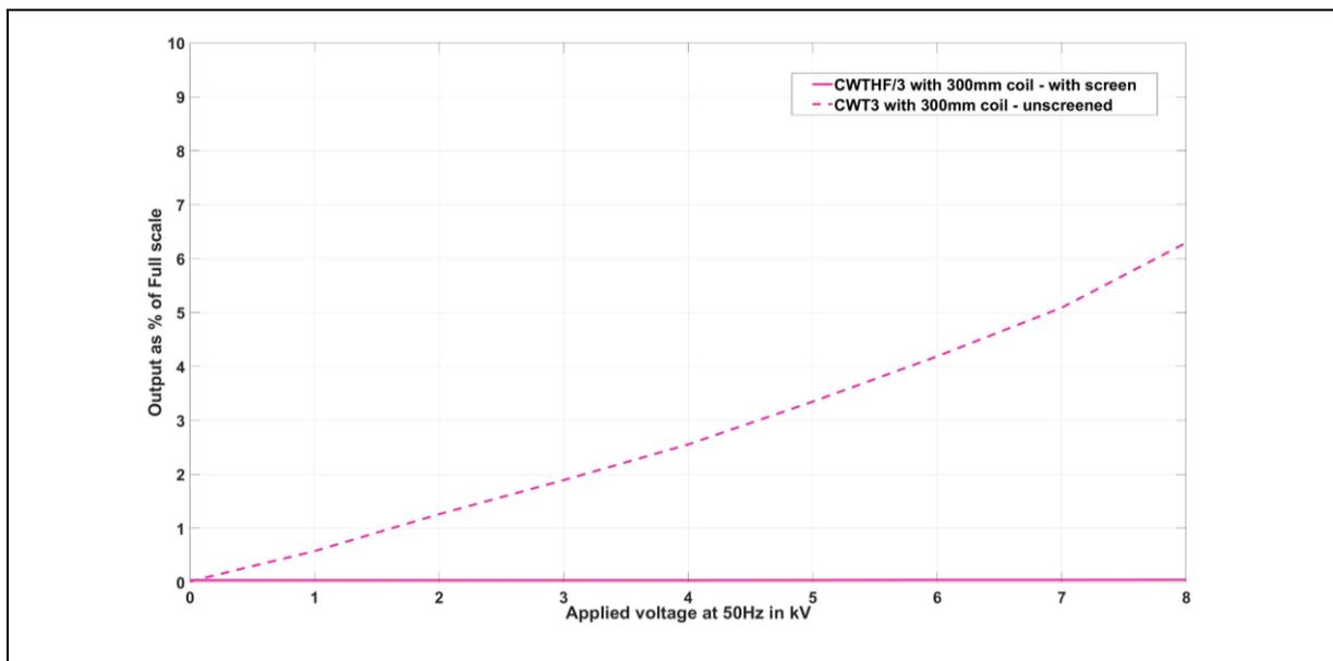
**Figure 8. Applying 0 to 8kVrms on a close coupled surface to the Rogowski coil, Coupled capacitance  $C_x = 23pF$**
