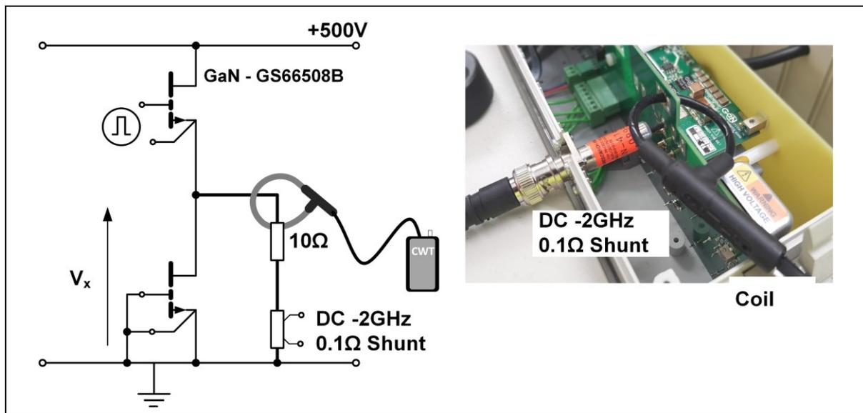
Figure 4. Fast switching circuit
