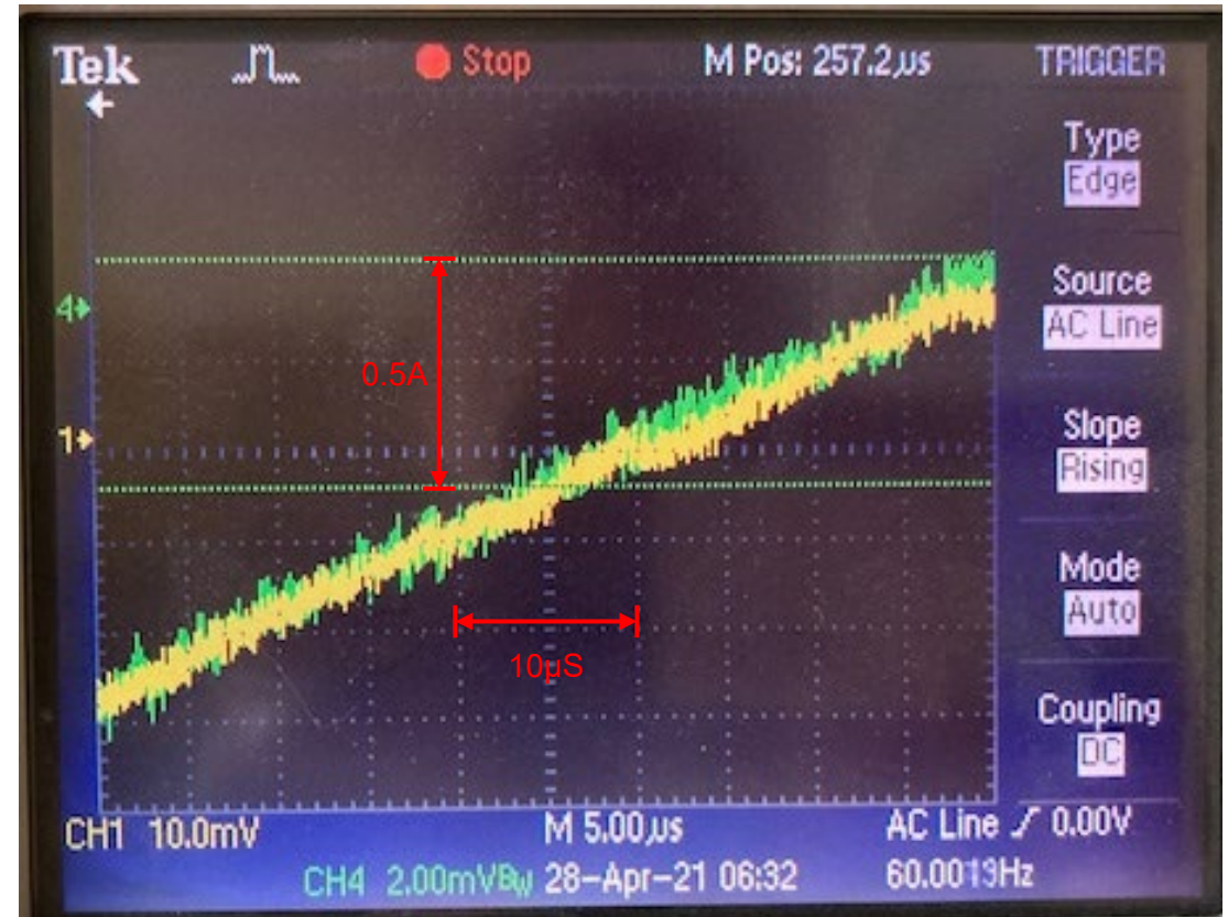
Fig 2: CPC \pm 250\text{A} fs as in Fig 1 but with high vertical sensitivity. No measurable zero crossing shift at 5\mu\text{s}/\text{div} .
