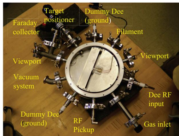
Figure 2: Vacuum chamber, ports, filament, and dee electrodes.
