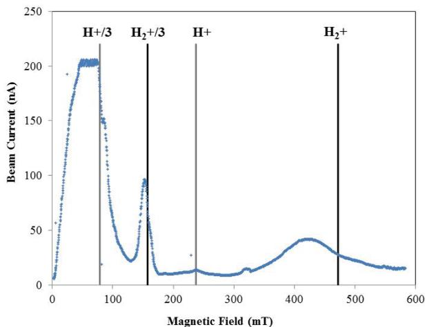
Figure 6: Highest current peak recorded, nearly 0.1 A, at 3.62 MHz, for hydrogen at approximately  $1 \times 10^{-4}$  Torr.
