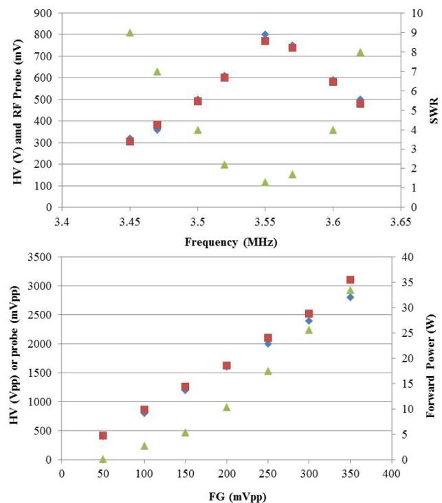
Figure 3: Tune at a frequency of 3.55 MHz. (Top) The peak-to-peak Dee voltage (blue diamond), RF pickup voltage (red square) and Standing-wave ratio (SWR) (green triangle) are plotted as a function of driving frequency. (Bottom) The peak-to-peak Dee and RF pickup voltages (symbols as above), and forward RF power (green triangles) are plotted as a function of peak-to-peak voltage from the function generator.
