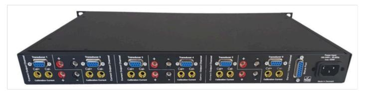
All above transducers do work with the DSSIU-6-1U, and the calibration current can be individually applied via the yellow 4mm banana plugs on the rear side. By putting the windings in series, up to six DCCT's can be calibrated at the same time with the same current.
