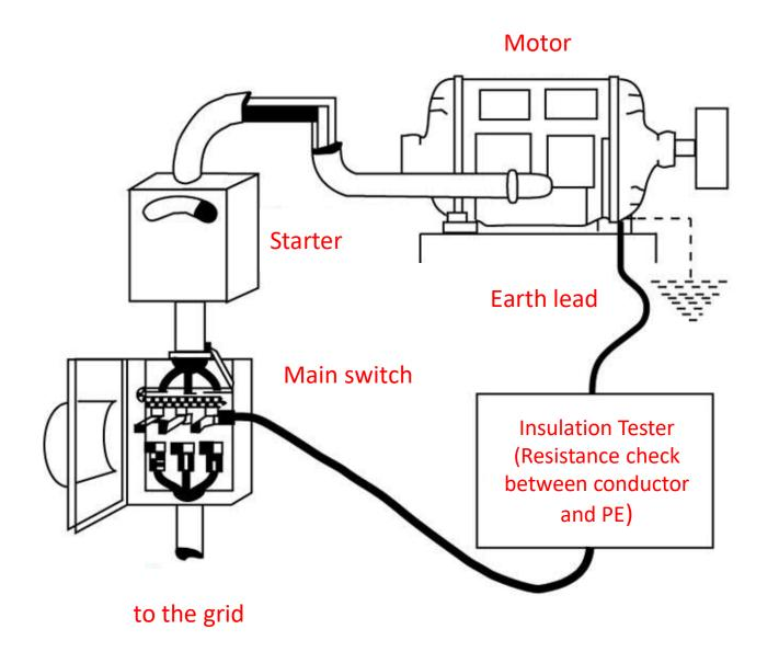
The insulation resistance must be measured between each active conductor and the protective conductor or earth.
