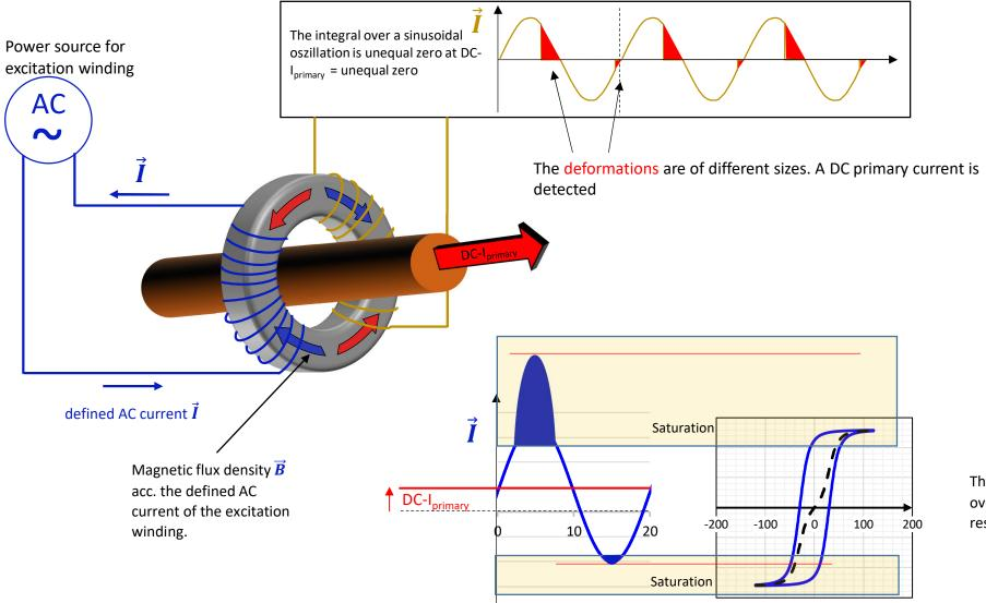
The magnetic flux density  $\vec{B}$ , averaged over a complete sinusoidal oscillation, results in zero.
