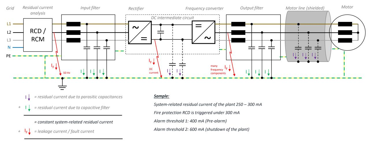
= measured total residual current of the RCM device
