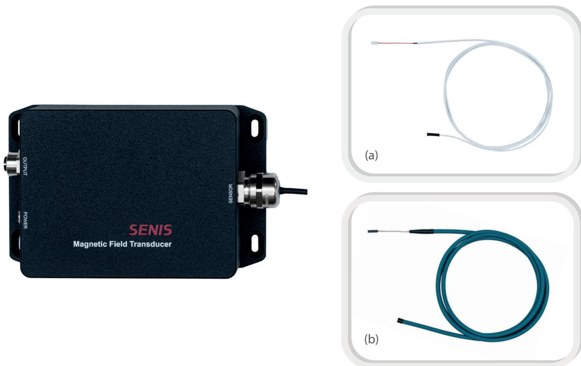
**Figure 2:** Photos of the 3-axis magnetic field transducers F3A with fully integrated 3-axis Hall Probe. Two cable variants are available: (a) white (thin) cable, OD 1.7 mm; (b) blue-marine (thick) cable, OD 6.5 mm.
