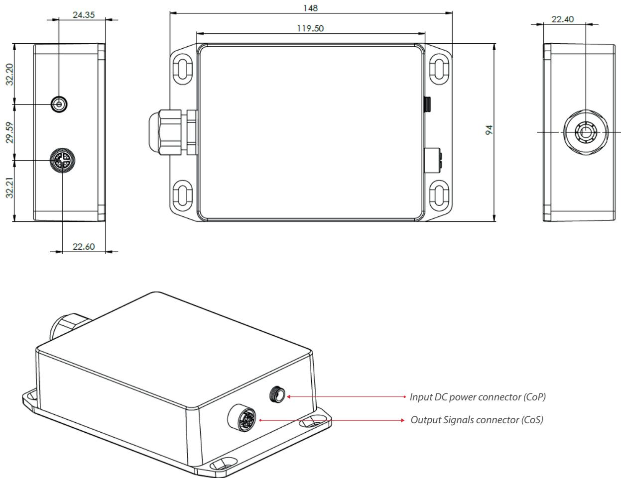
**Figure 4:** Structure and dimensions of the new 3-channel analogue electronic module allowing for firm connection of a Hall probe.
