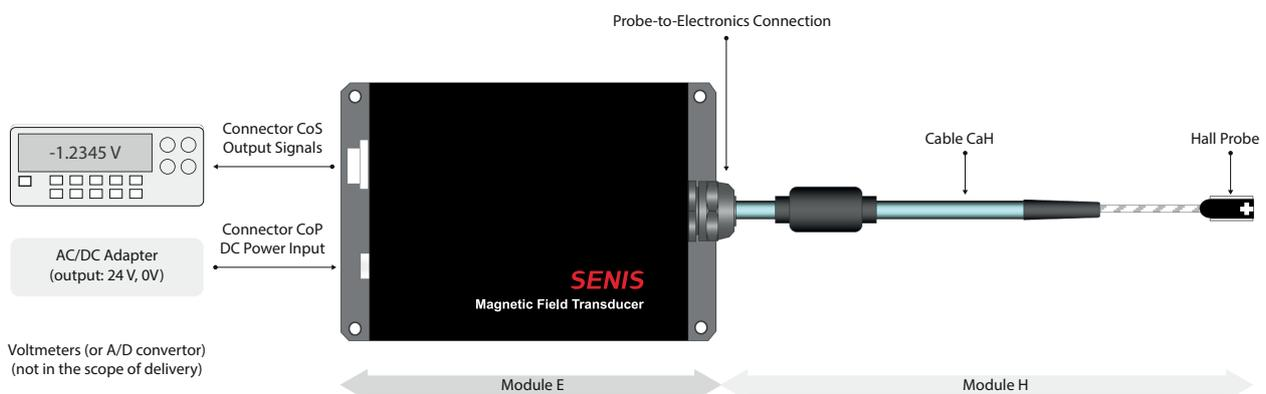
**Figure 1:** Typical measurement setup with a SENIS magnetic-field-to-voltage transducer with fully integrated Hall Probe (Module H) and Electronic (Module E)
