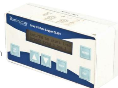
The Data Logger measures the magnetic gradient during surveys using a high sampling rate, with automatic averaging for each reading. Sampling rate can be adjusted to suit the operator's pace.
