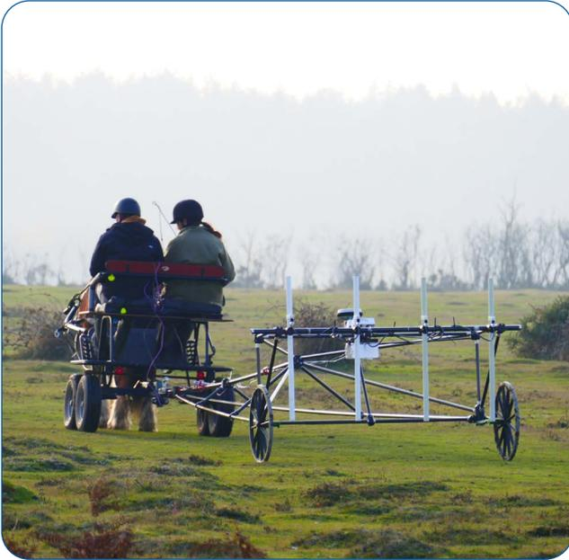
The Grad601 is a fluxgate gradiometer, used for measuring minute variations in the magnetic field that are caused by hidden anomalies in the ground such as archaeological and geophysical features, pipes, cables, waste drums, unexploded ordnance, and other signs of human activity.
