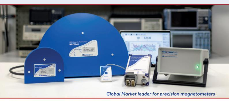
Launched 25 years ago, Metrolab's NMR Magnetic Field Cameras expedite field mapping for Magnetic Resonance Imaging (MRI) magnets. They reduce acquisition times from hours to minutes, positioning errors to fractions of a millimeter, and they render human and drift errors negligible.
