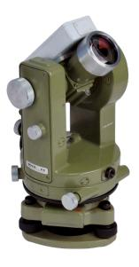
As these optical theodolites are no longer manufactured, each unit supplied is pre-used, restored as far as possible to its original condition and meticulously converted to be steel-free. All magnetic components are replaced by a non-magnetic equivalent. The horizontal and vertical axis bearings are replaced with specially plated phosphor bronze parts, and the steel ball-race removed from the horizontal axis. The WILD axis lubrication system ensures that these parts require zero maintenance.
