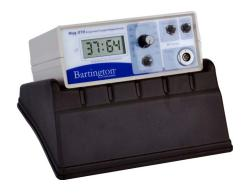
This battery powered instrument provides the drive for the probe and processes its output to show the field strength on a 4½-digit display, updated at 2 readings per second. An analogue output is also provided. The Mag-01H may be fitted with an audio output indicator, on request. This facility enables the operator to seek the null position without continuously monitoring the digital display. A sensitivity switch can be used to select 1nT or 0.1nT resolution.
