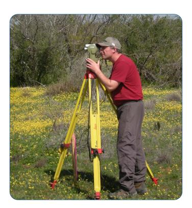
The Mag-01H Declinometer/Inclinometer system provides fast, accurate and convenient measurements of the declination and inclination of the geomagnetic field.
