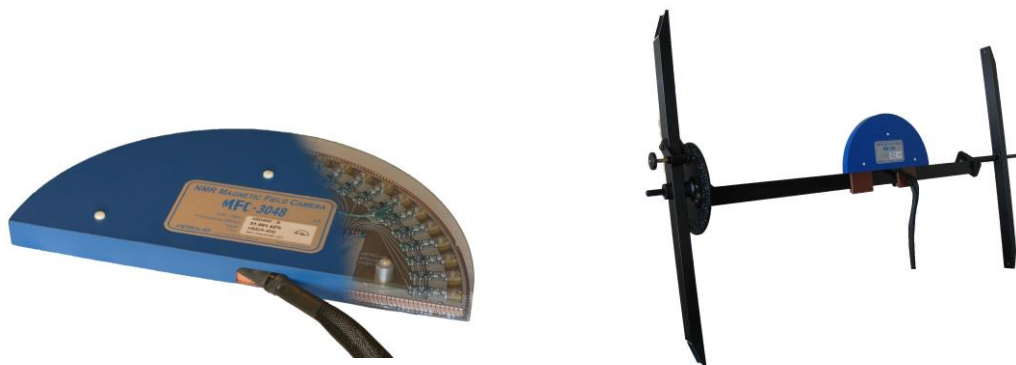
Figure 5. The Magnetic Field Camera probe array: (a) cut-away showing the probe positions; (b) as installed in a horizontal MRI magnet.
