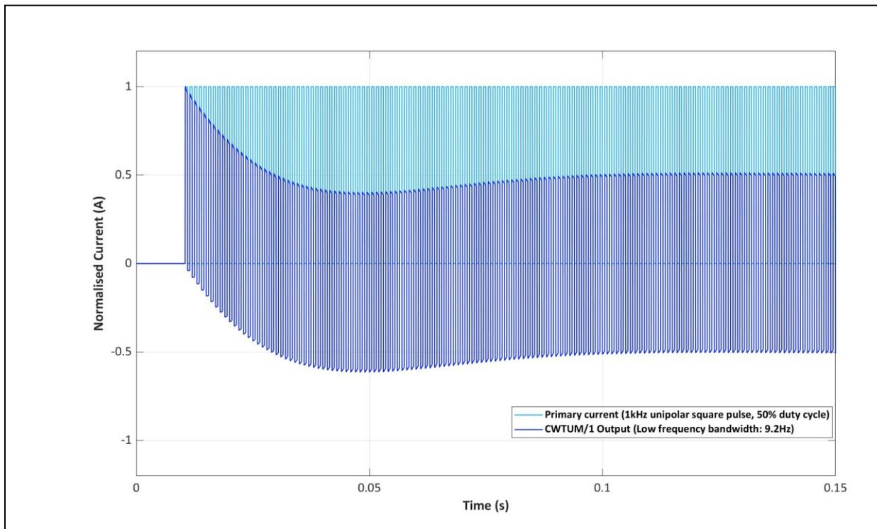
**Figure 7. Typical settling period for a unipolar pulse-train**
