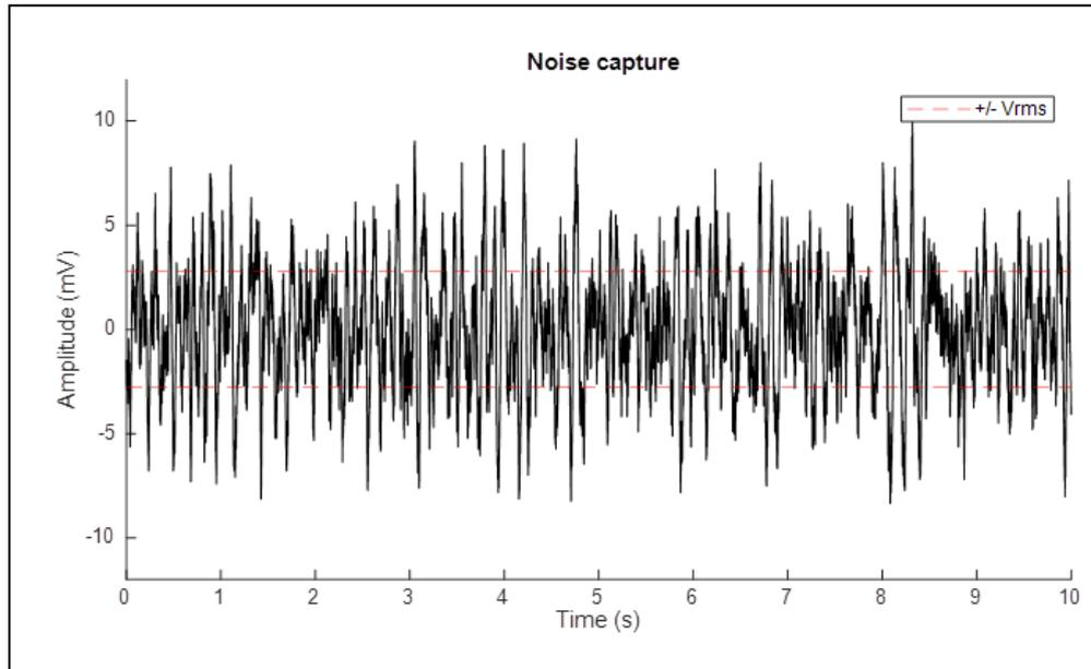
**Figure 4. Noise capture of the CWTUM/1 (RMS = 2.4mV)**
