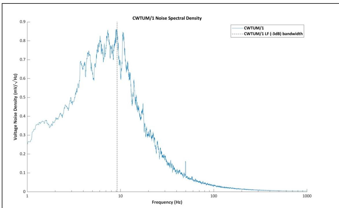
**Figure 3. Voltage noise distribution of the CWTUM/1**
