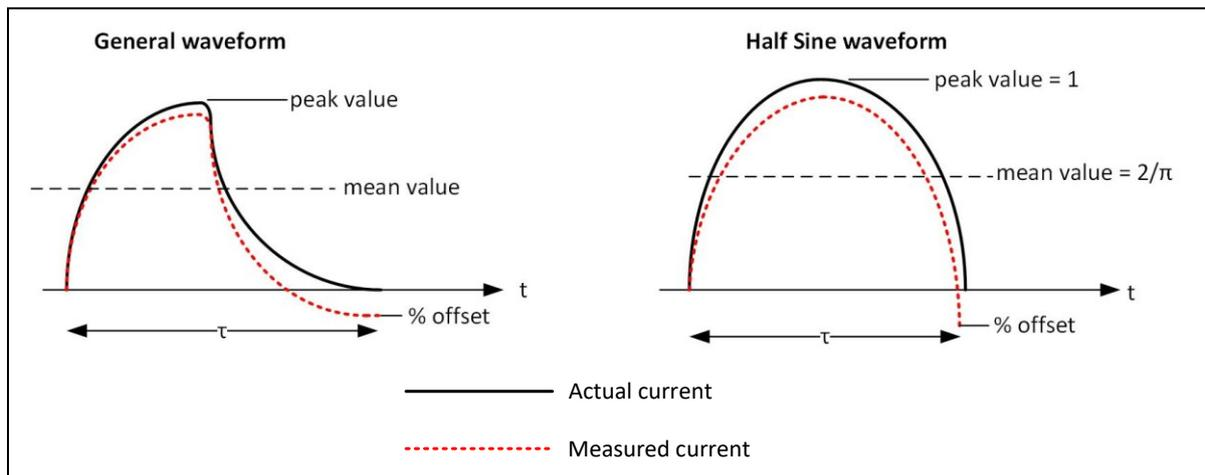
**Figure 6. Droop calculation for any pulse where  $\tau \ll T$**
