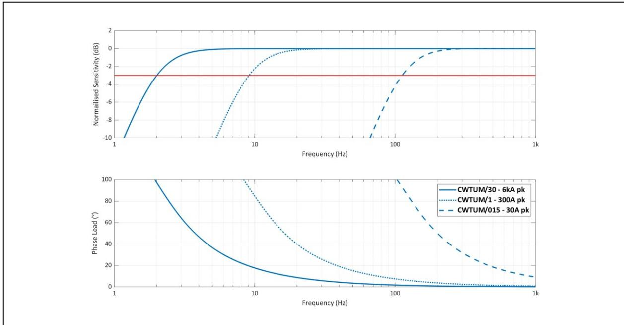
**Figure 2. Theoretical Low frequency bandwidth of the CWTUM product range reduces as the current rating increases**
