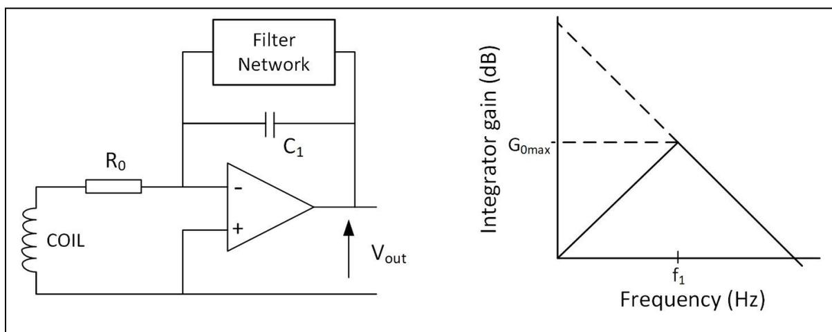
**Figure 1. Simplified integrator block diagram and an illustration of the maximum integrator gain and low frequency roll off**
