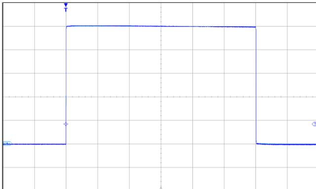
Ch 1: Co-axial shunt - DC-2GHz
