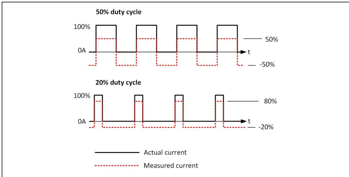
*Figure 8. Measured offset of a unipolar pulse-train (after settling)*
