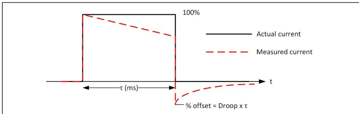
**Figure 5. Droop definition - based on a rectangular pulse**
