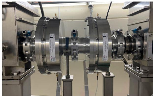
Figure 1: Resonating cavities installed at PROSCAN.
