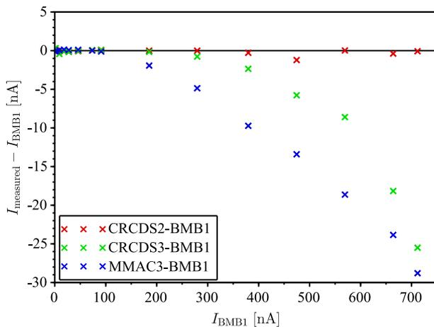
Figure 4: Differences of currents measured by BMB1 and CRCDS2 (red), CRCDS3 (green) and MMAC3 (blue).
