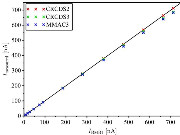
Figure 3: Currents measured by CRCDS2 (red), CRCDS3 (green) and MMAC3 (blue) versus BMB1.
