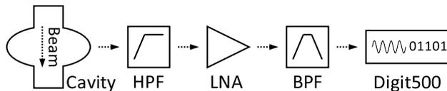
Figure 2: Schematic of the CRCDS measurement chain.
