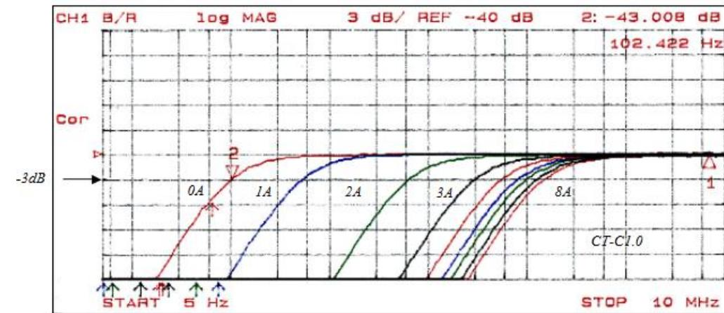
Lower cut-off frequency dependence to DC primary current
