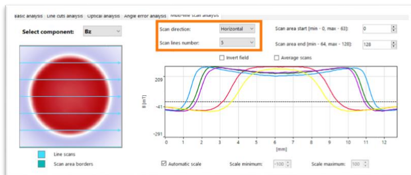
Figure 16: SENIS Vision software with visualization of the horizontal multi-line measurement results
